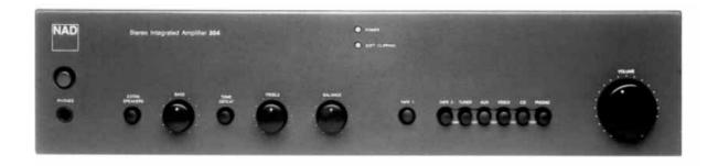
The 304 essentially extends the 302 with power increased to 35 watts per channel into 8 ohms and generous headroom permitting untroubled peaks of 120 watts per channel.
